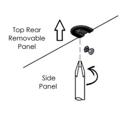
2 Screw Female and Male connectors into the pilot holes provided on both sides as shown below for wedge position.
