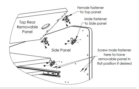
Push evenly by holding the panel from the grommet holes. The fasteners will lock together. Pull in the same manner to remove the panel.
